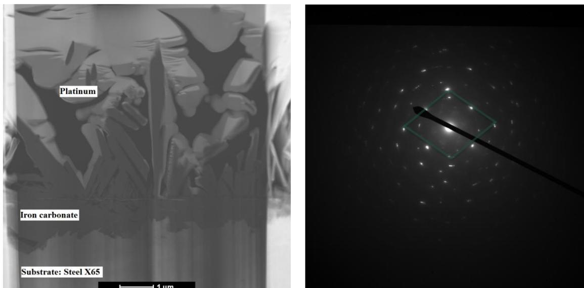
**Figure 8: TEM image and ED data of the plates found on the X65 mild steel before the addition of undissociated acetic acid.**
